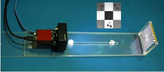
Figure 5. Plexiglas mount with camera, ring lighting and Siemens star target. The small image in the middle shows the second pattern with different colored areas and photogrammetric targets.
