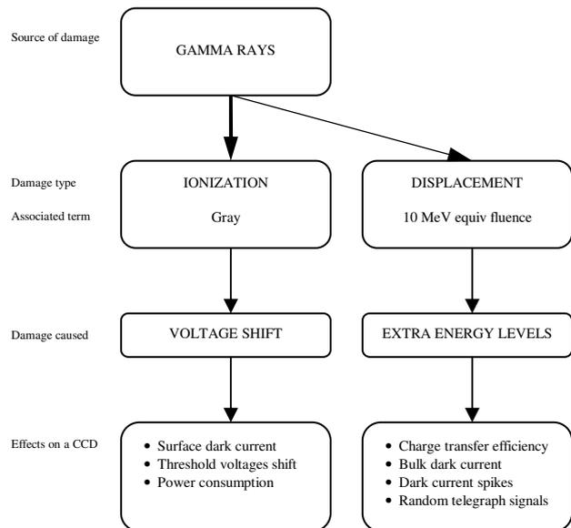
Figure 1. The radiation damage tree for CCDs. Illustration from (Bassler, 2004)
