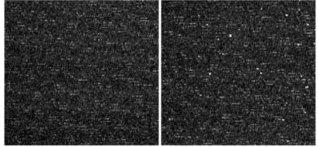
Figure 6. Section from images without radiation (left) and with 100 mSv/h gamma radiation (right). Histograms are stretched to make “hot pixels” visible.
